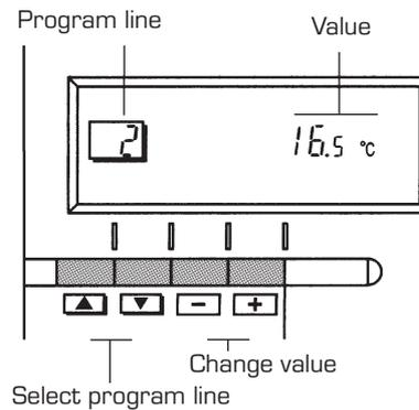
As soon as the cover is open, the display and the key functions are switched on. The number in the square represents the programme lines that may be selected with the arrow keys.
