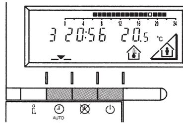
The operating mode desired is selected by pressing the relative key with the corresponding symbol. The choice is displayed with the symbol
