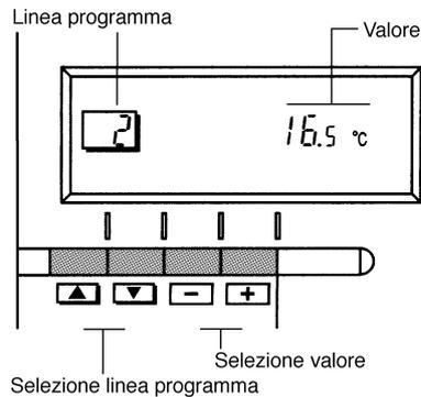
As soon as the cover is open, the display and the key functions are switched on. The number in the square represents the programme lines that may be selected with the arrow keys.
