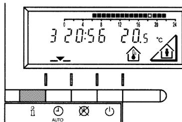
For every operation of the Info key the following list of items, one after the other, are displayed. The thermosensor continues to function independently of the display.
