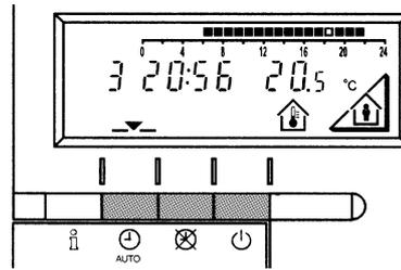
The operating mode desired is selected by pressing the relative key with the corresponding symbol. The choice is displayed with the symbol
